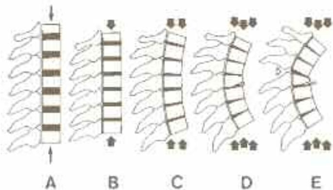
**Figure 5:** (A) Axial loading of the cervical spine (B) first results in compressive deformation of the intervertebral discs. As the energy input continues and maximum compressive deformation is reached, angular deformation and buckling occur (C). The spine fails in a flexion mode, with resulting fracture, dislocation, or sub-luxation (D and E).
